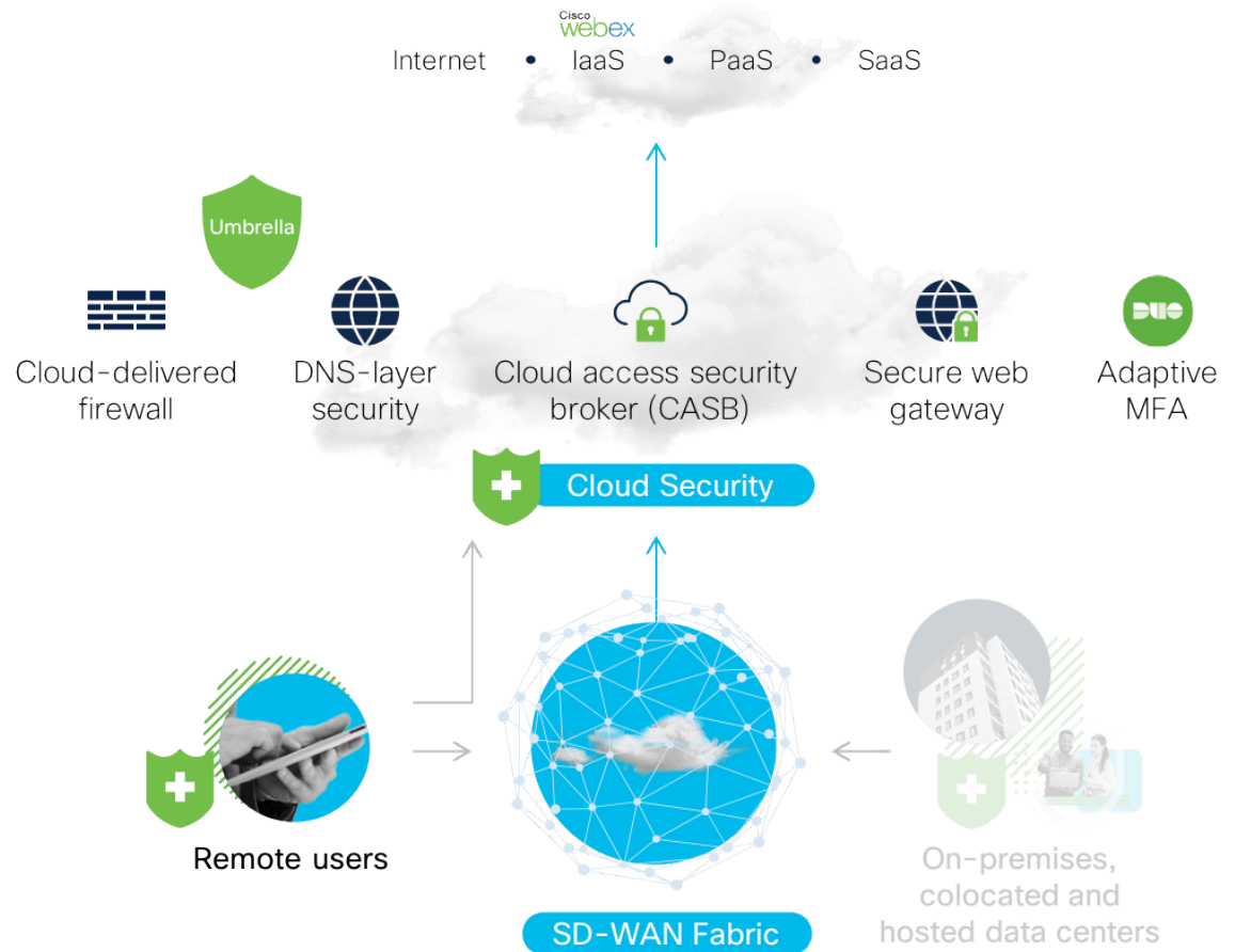
Figure 2: Cisco secure remote access architecture.
